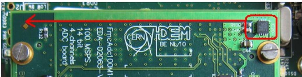
5. 47 Ohm & 56 Ohm resistors (matching input impedance to 50 Ohm, right behind the SMC connectors) in 2512 package (available in Farnell for ex.)
