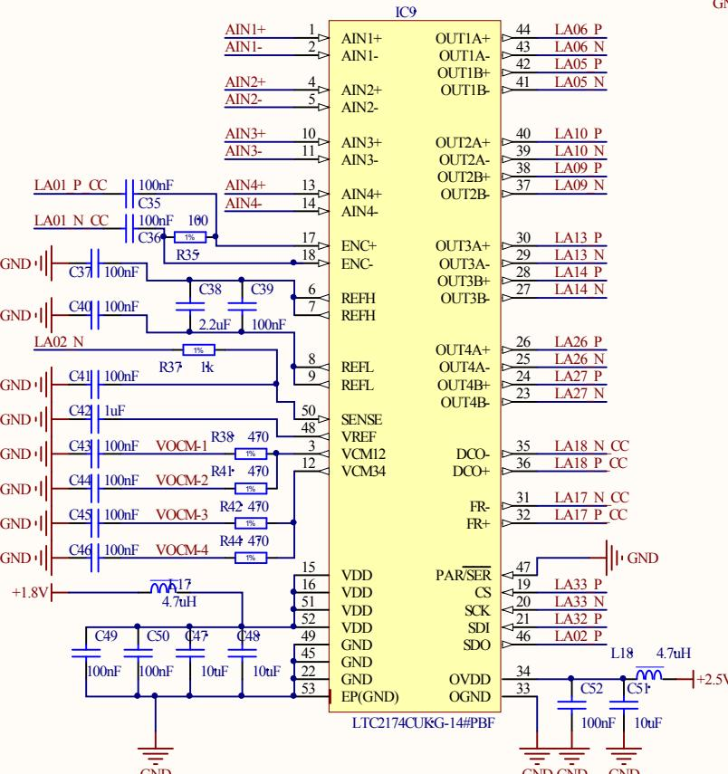
CC postfix lines are used as clocklines - in the spec, there is a note, that they can be used as a clock lines for synchronous applications.
