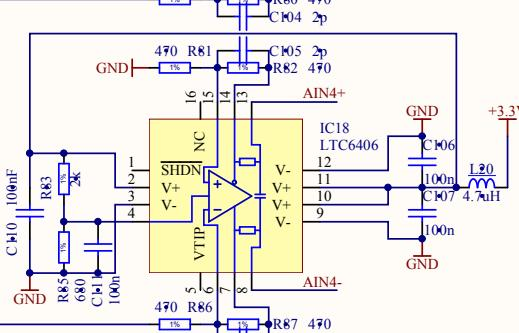
resistor divider creates potential of 0.9V for VOCM inputs (common mode output potential)
