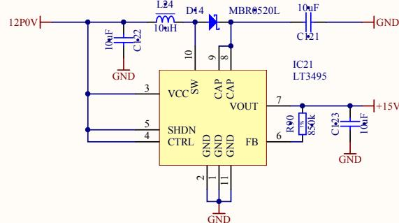
△ standard low noise boost converter. According to the datasheet, output ripple approx. 10mV
