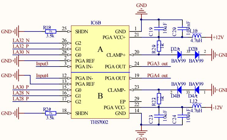
BAV99 diodes clamp the output of the PGA and therefore don't allow the next stage to be deeply saturated
