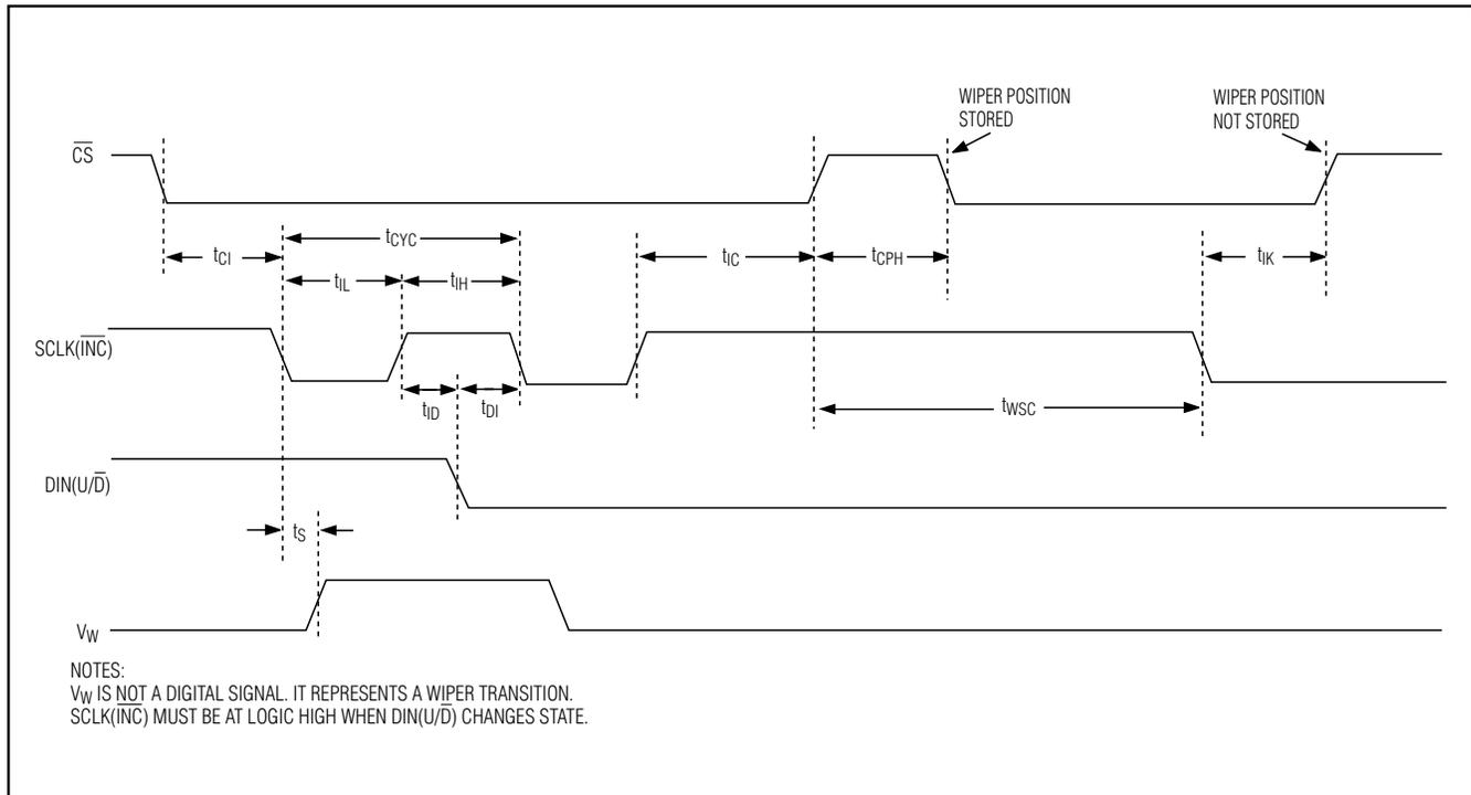
Figure 8. Up/Down Serial-Interface Timing Diagram ( $SPI/UD = 0$ )
