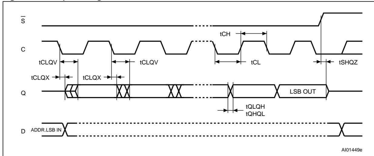
Figure 24.  $V_{PPH}$  timing
