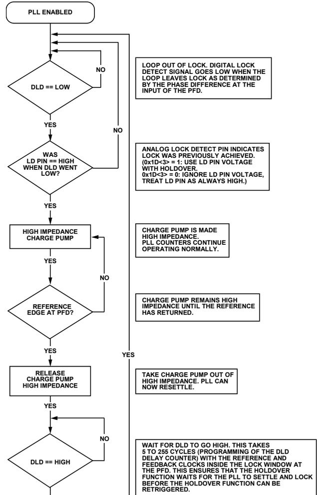
Figure 51. Flow Chart of Automatic/Internal Holdover Mode
