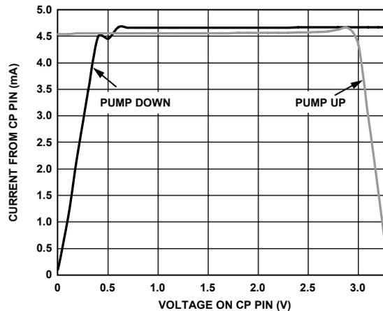
Figure 11. Charge Pump Characteristics @  $V_{CP} = 3.3 V$
