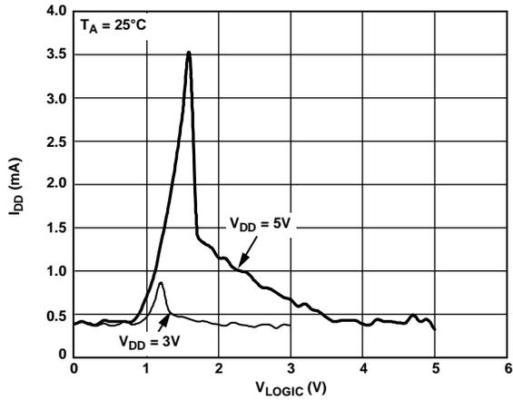
Figure 24. Supply Current vs. Logic Input Voltage
