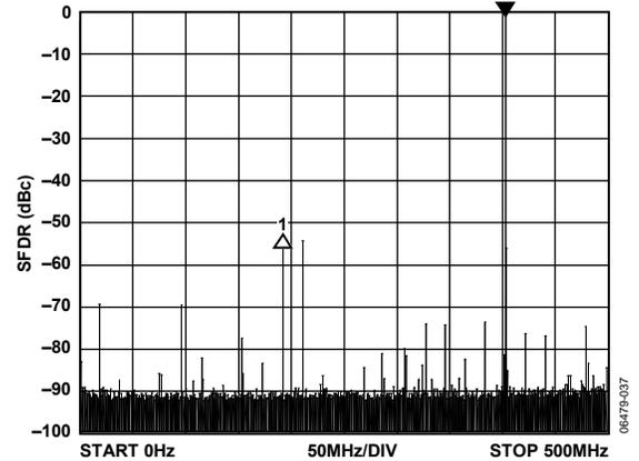
Figure 11. Wideband SFDR at 403 MHz, REFCLK = 1 GHz
