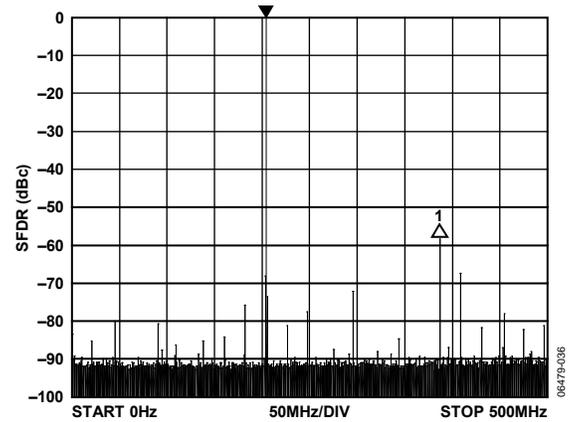
Figure 10. Wideband SFDR at 204 MHz, REFCLK = 1 GHz
