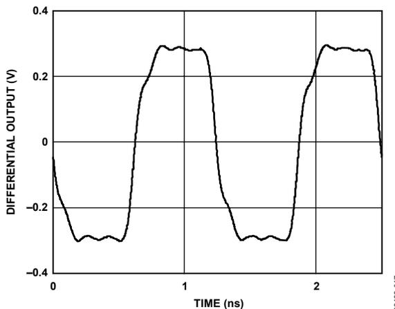
Figure 22. LVDS Output (Differential) @ 800 MHz
