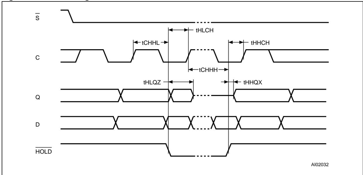
Figure 23. Output timing
