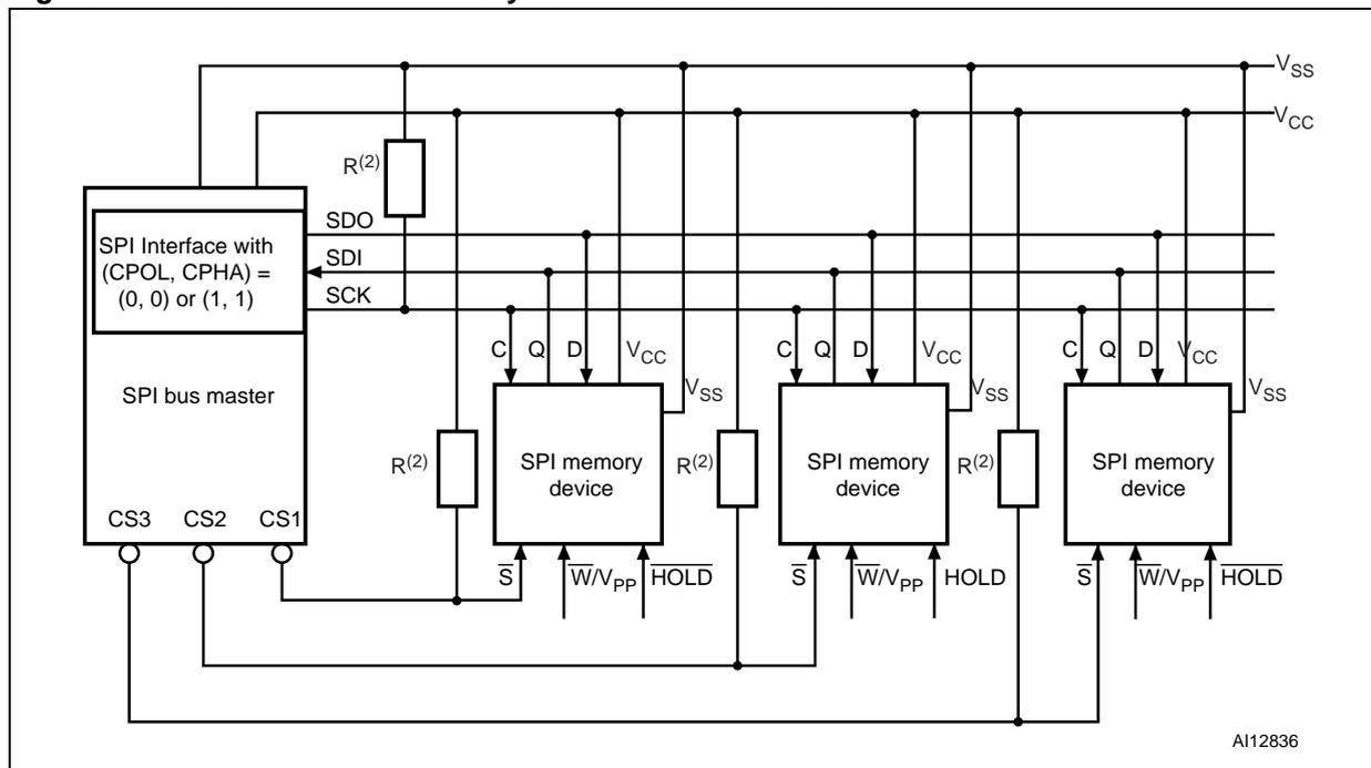
1. The Write Protect ( $\overline{W}/V_{PP}$ ) and Hold ( $\overline{HOLD}$ ) signals should be driven, High or Low as appropriate.
