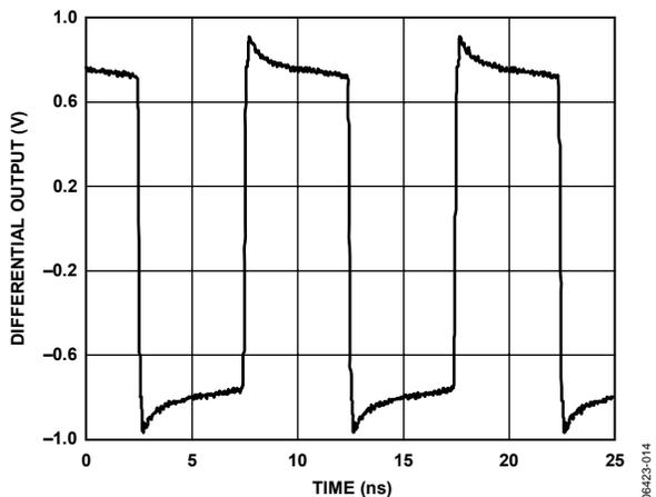
Figure 19. LVPECL Output (Differential) @ 100 MHz
