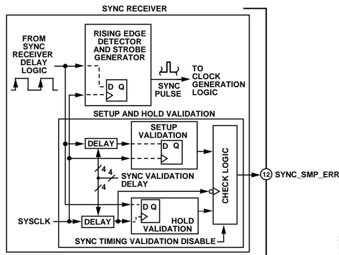
Figure 54. Sync Timing Validation Block
