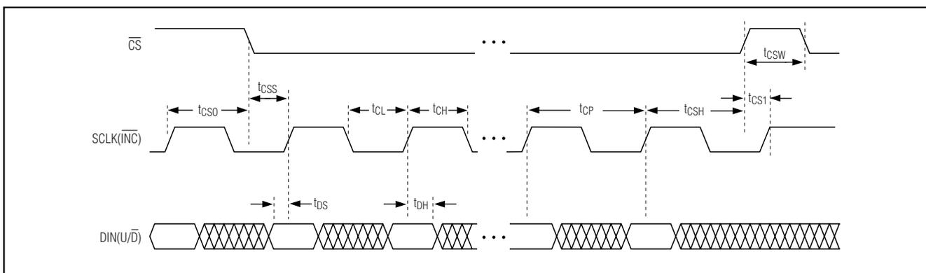
Figure 3. SPI-Compatible Serial-Interface Timing Diagram (SPI/UD = 1)
