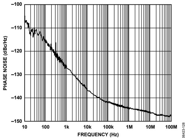
Figure 33. Phase Noise (Additive) LVPECL @ 1600 MHz, Divide-by-1
