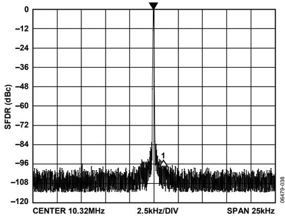
Figure 12. Narrow-Band SFDR at 10.32 MHz, REFCLK = 1 GHz
