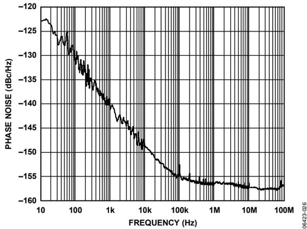
Figure 31. Phase Noise (Additive) LVPECL @ 245.76 MHz, Divide-by-1
