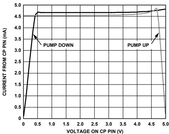
Figure 12. Charge Pump Characteristics @  $V_{CP} = 5.0 V$
