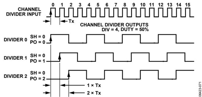
Figure 53. Effect of Coarse Phase Offset (or Delay)
