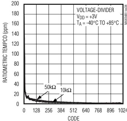
**VARIABLE-RESISTOR TEMPERATURE COEFFICIENT vs. CODE**
