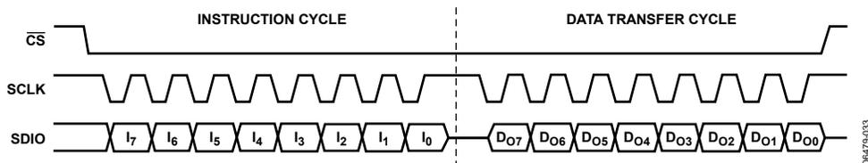
Figure 58. 2-Wire Serial Port Read Timing, Clock Stall High
