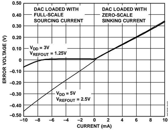
Figure 18. Headroom at Rails vs. Source and Sink
