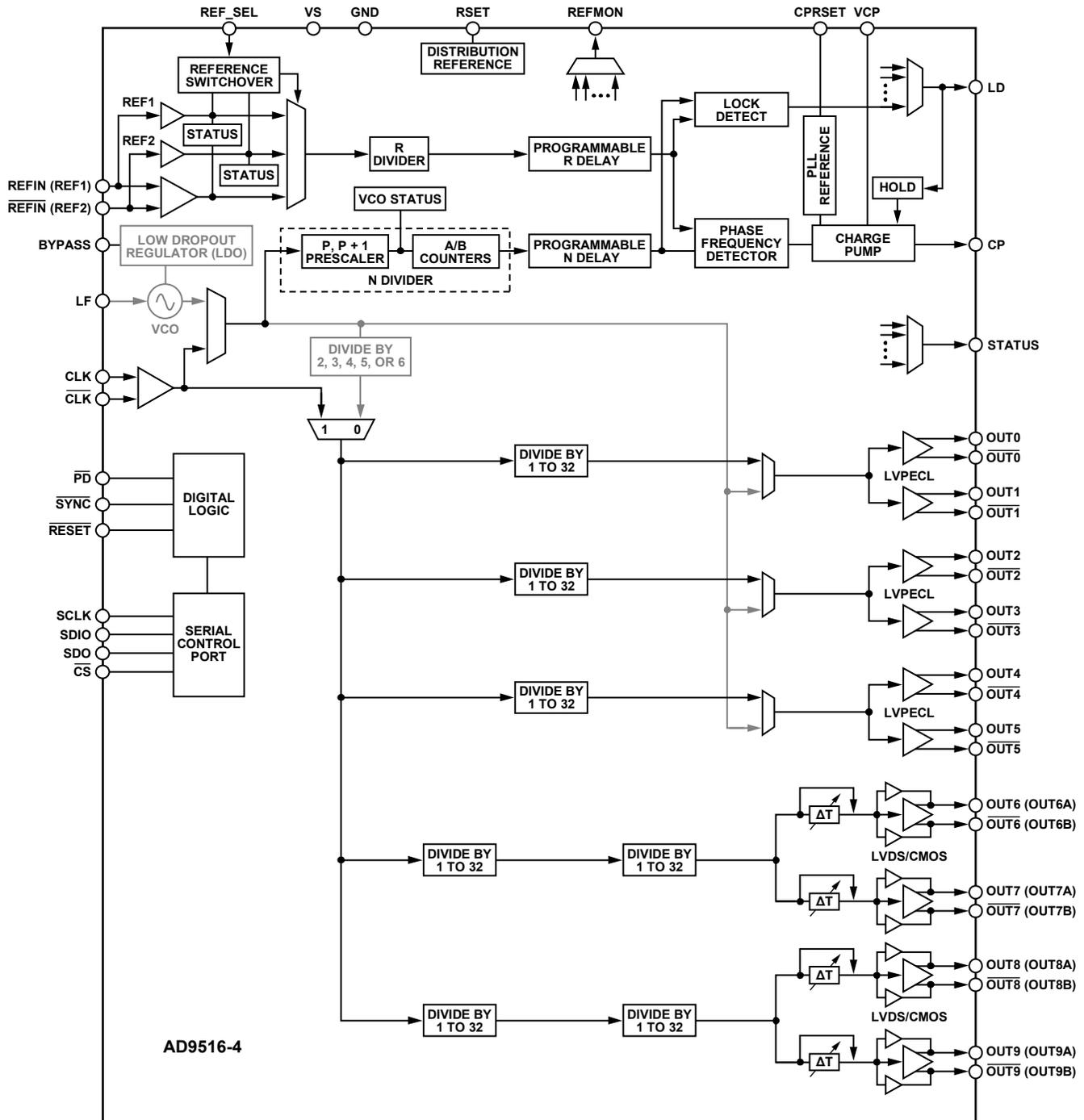
Figure 44. Clock Distribution or External VCO < 1600 MHz
