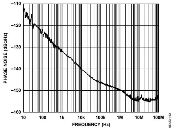
Figure 34. Phase Noise (Additive) LVDS @ 200 MHz, Divide-by-1
