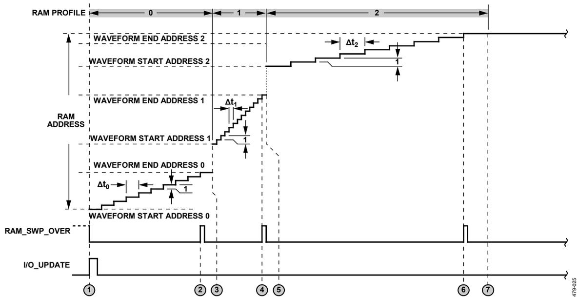
Figure 44. Internal Profile Control Timing Diagram (Burst)
