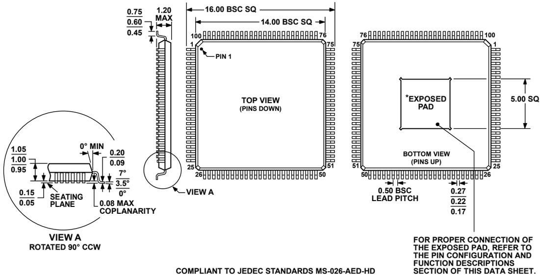
Figure 59. 100-Lead Thin Quad Flat Package, Exposed Pad [TQFP\_EP] (SV-100-4)
