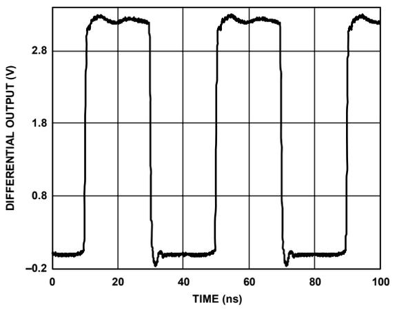
Figure 23. CMOS Output @ 25 MHz
