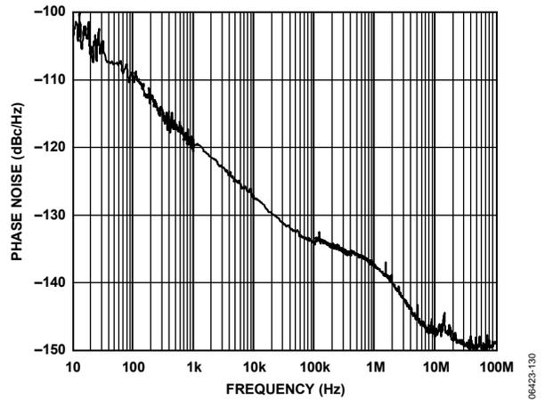
Figure 35. Phase Noise (Additive) LVDS @ 800 MHz, Divide-by-2
