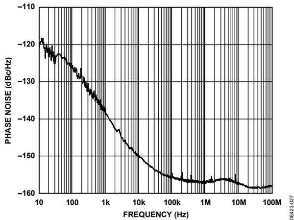
Figure 32. Phase Noise (Additive) LVPECL @ 200 MHz, Divide-by-5
