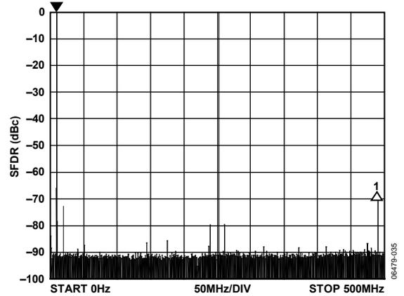
Figure 9. Wideband SFDR at 10 MHz, REFCLK = 1 GHz
