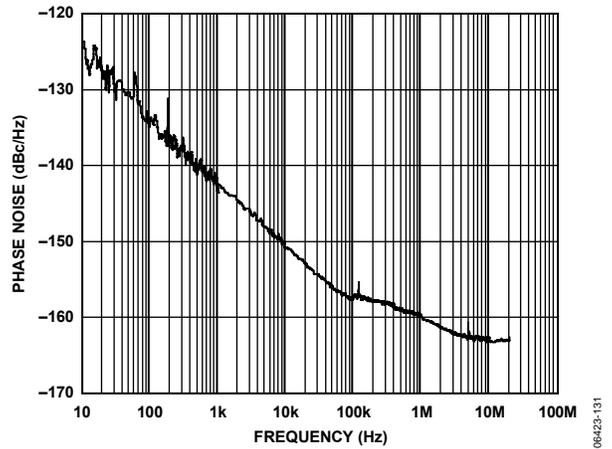
Figure 36. Phase Noise (Additive) CMOS @ 50 MHz, Divide-by-20
