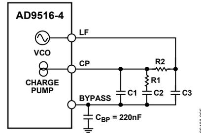
Figure 46. Example of External Loop Filter for PLL
