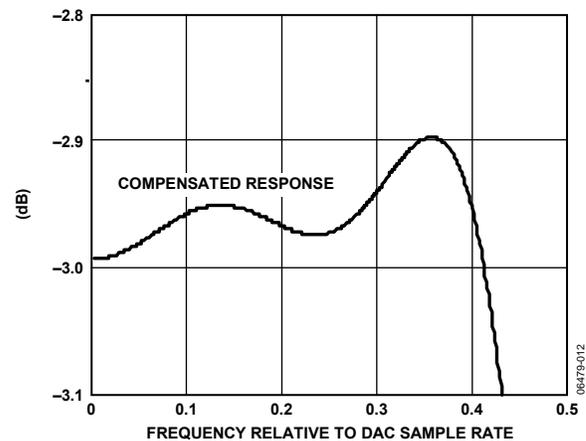
Figure 29. DAC Response with Inverse Sinc Compensation
