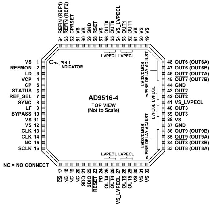
Figure 6. Pin Configuration
