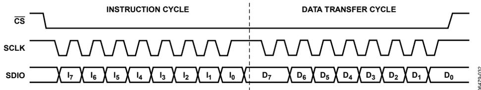
Figure 57. Serial Port Write Timing, Clock Stall High
