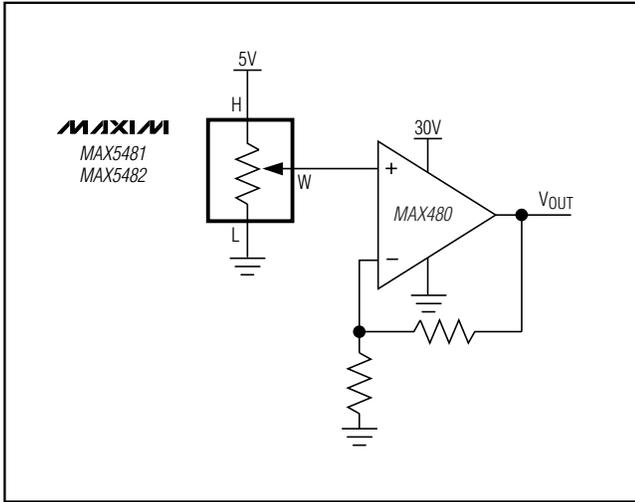
Figure 9. Positive LCD Bias Control Using a Voltage-Divider
