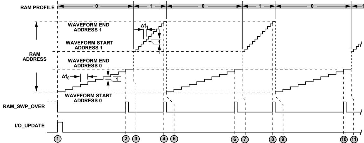
Figure 45. Internal Profile Control Timing Diagram (Continuous)
