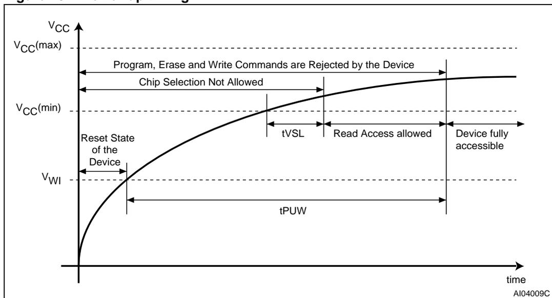
Table 8. Power-up timing and  $V_{WI}$  threshold for 65 nm devices<sup>(1)</sup>
