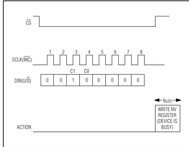
Figure 6. Copy Wiper Register to NV Register Operation
