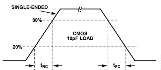
Figure 5. CMOS Timing, Single-Ended, 10 pF Load
