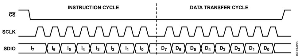
Figure 55. Serial Port Write Timing, Clock Stall Low
