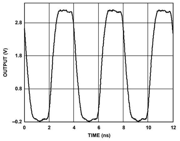
Figure 24. CMOS Output @ 250 MHz
