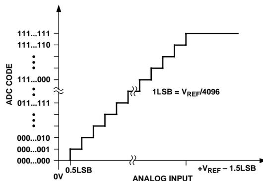
Figure 7. Transfer Characteristic
