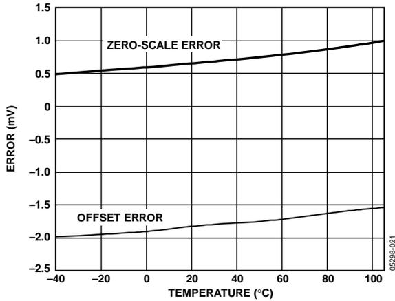
Figure 13. Zero-Scale Error and Offset Error vs. Temperature
