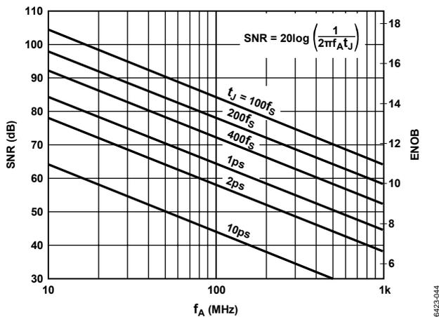
Figure 68. SNR and ENOB vs. Analog Input Frequency
