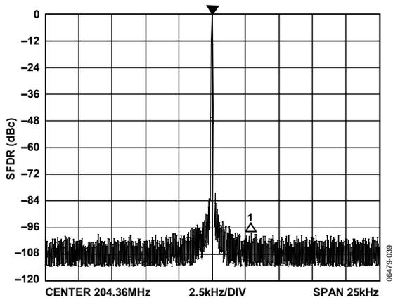
Figure 13. Narrow-Band SFDR at 204.36 MHz, REFCLK = 1 GHz
