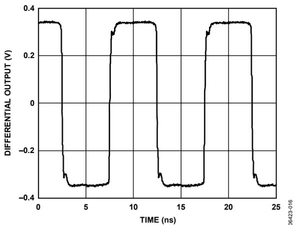
Figure 21. LVDS Output (Differential) @ 100 MHz
