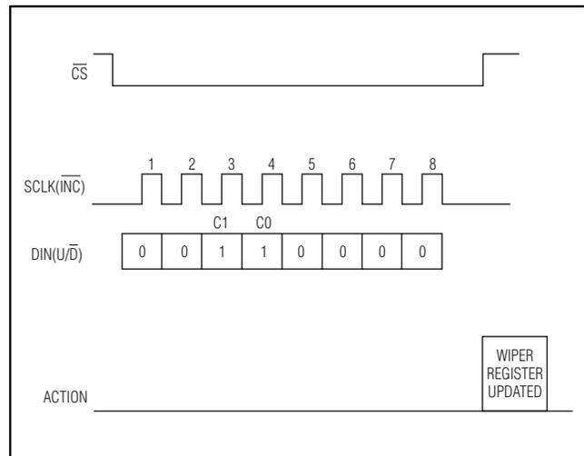
Figure 7. Copy NV Register to Wiper Register Operation
