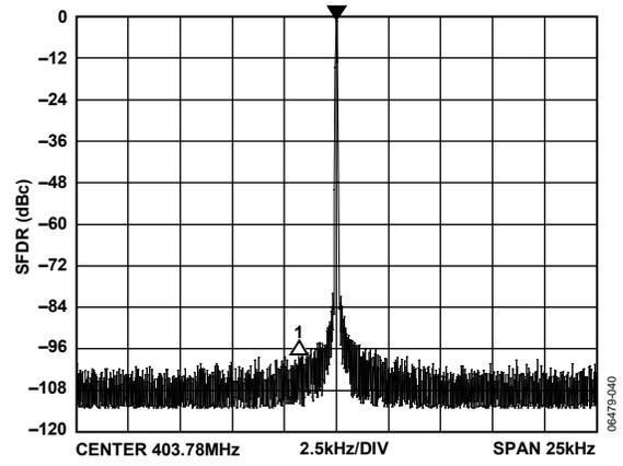
Figure 14. Narrow-Band SFDR at 403.78 MHz, REFCLK = 1 GHz
