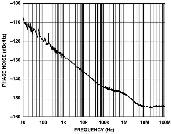
Figure 37. Phase Noise (Additive) CMOS @ 250 MHz, Divide-by-4
