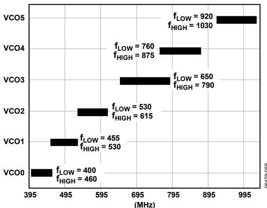
Figure 33. VCO Ranges Including Atypical Wafer Process Skew
