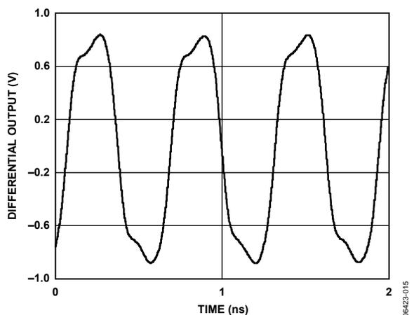
Figure 20. LVPECL Output (Differential) @ 1600 MHz
