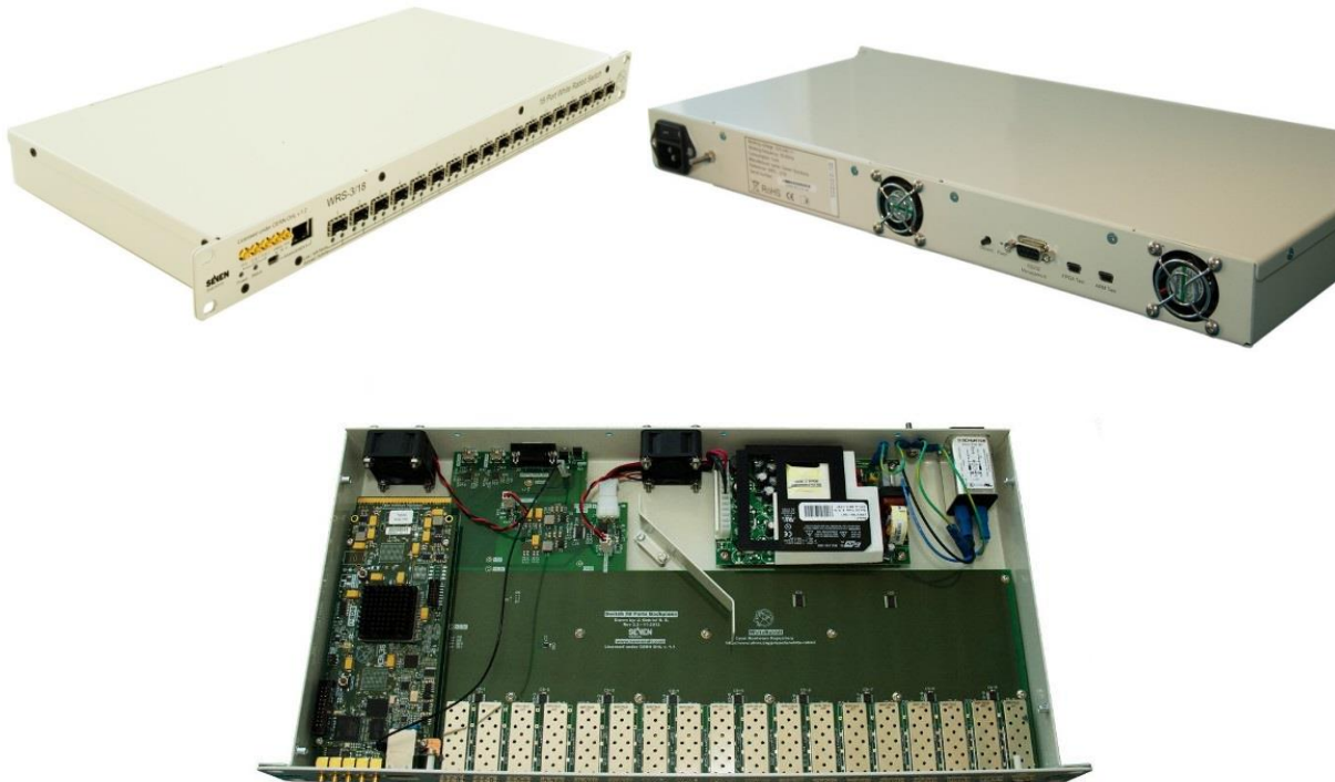
Figure 7: Front, back and inside views of the White Rabbit Switch
