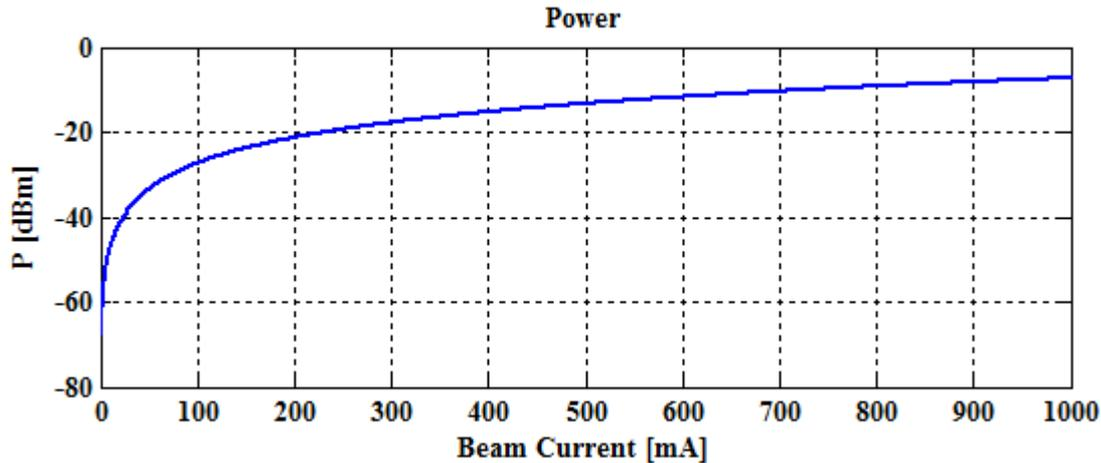
Figure 4: Signal characteristics on the input of the RFFE electronics as function of beam current for 500 MHz.
