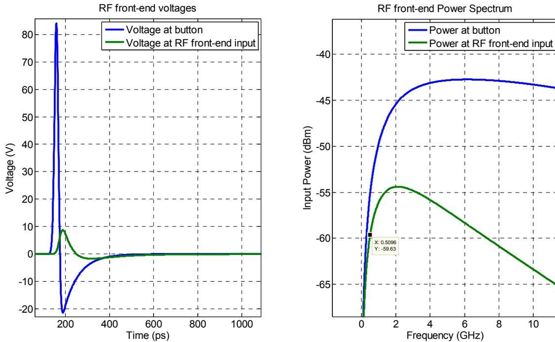
Figure 3: Time and frequency domain signal characteristics for the single-bunch mode of operation. The green curve is the signal after 25 meters of cables.
