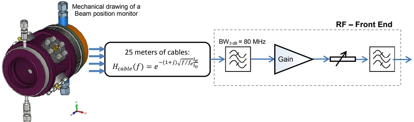
Figure 2: General block diagram that describes each of the four channels of the RFFE.
