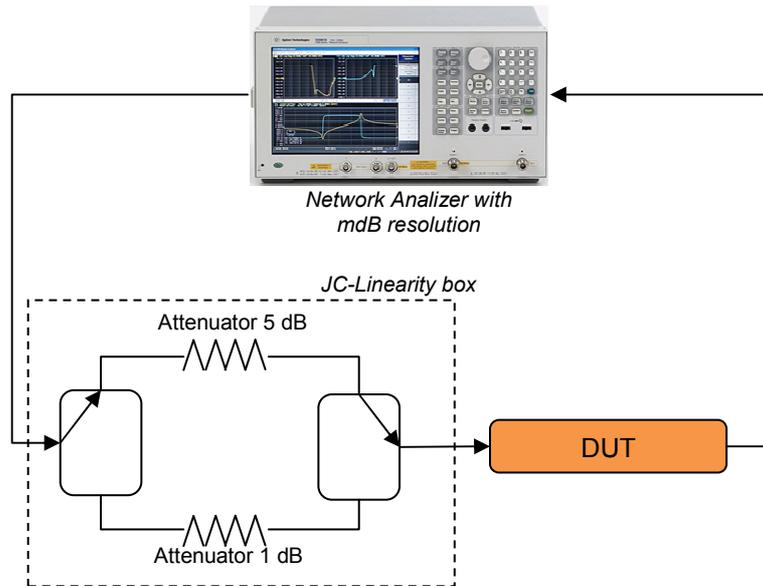
Figure 8: Scheme used to measure the linearity of active devices.
