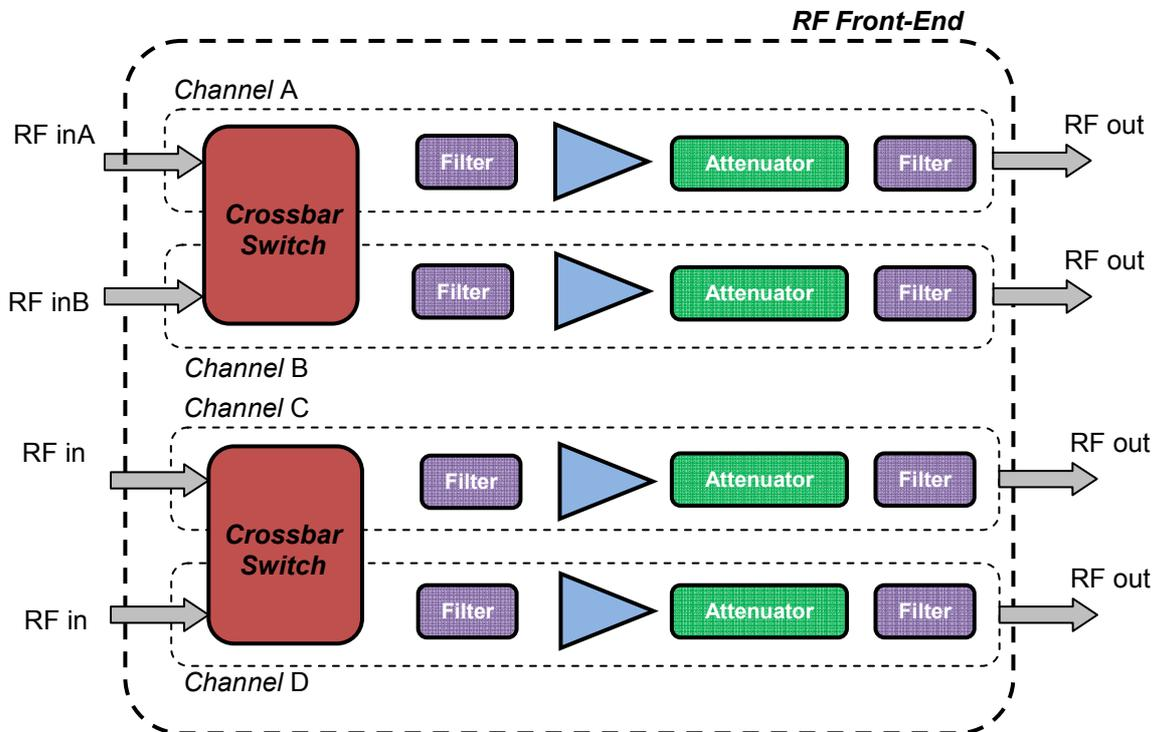
Figure 5: Diagram of the RFFE electronics.
