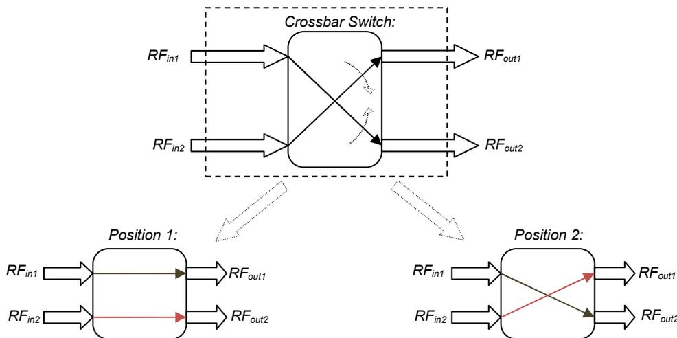
Figure 6: Crossbar switching scheme. The post-processing will correct the non-linearities from the measured signal using this *Crossbar switching scheme*.
