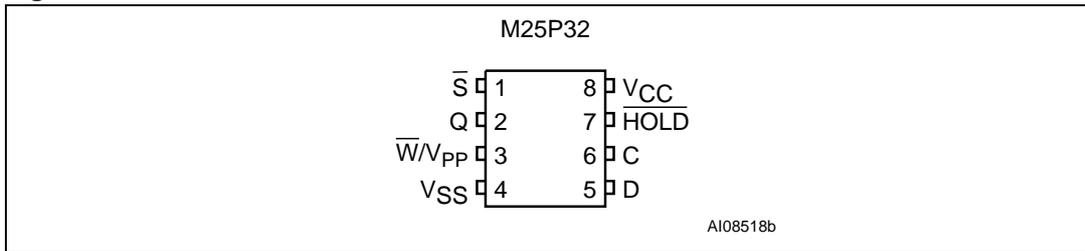
1. There is an exposed die paddle on the underside of the MLP8 package. This is pulled, internally, to V<sub>SS</sub>, and must not be allowed to be connected to any other voltage or signal line on the PCB.
