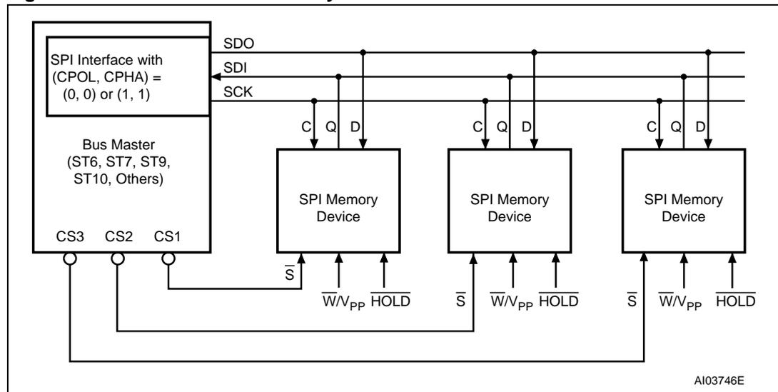
1. The Write Protect ( $\bar{W}/V_{PP}$ ) and Hold ( $\bar{HOLD}$ ) signals should be driven, High or Low as appropriate.
