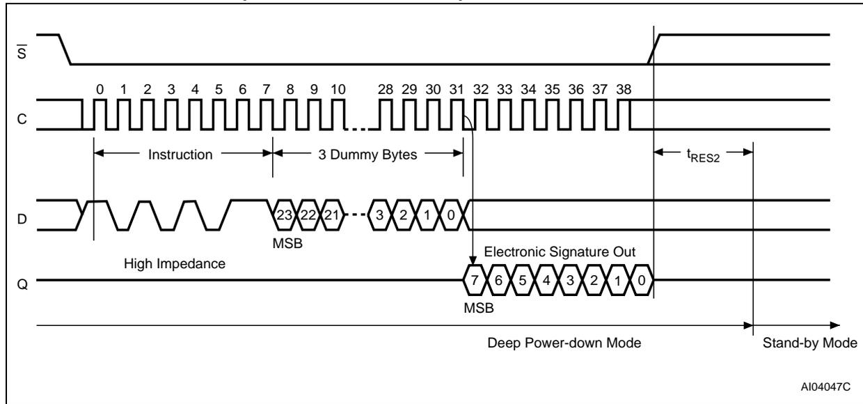
1. The value of the 8-bit Electronic Signature, for the M25P32, is 15h.
