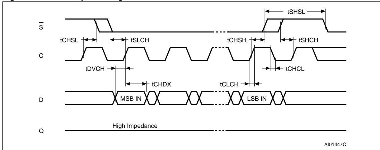
Figure 24. Write Protect Setup and Hold Timing during WRSR when SRWD=1
