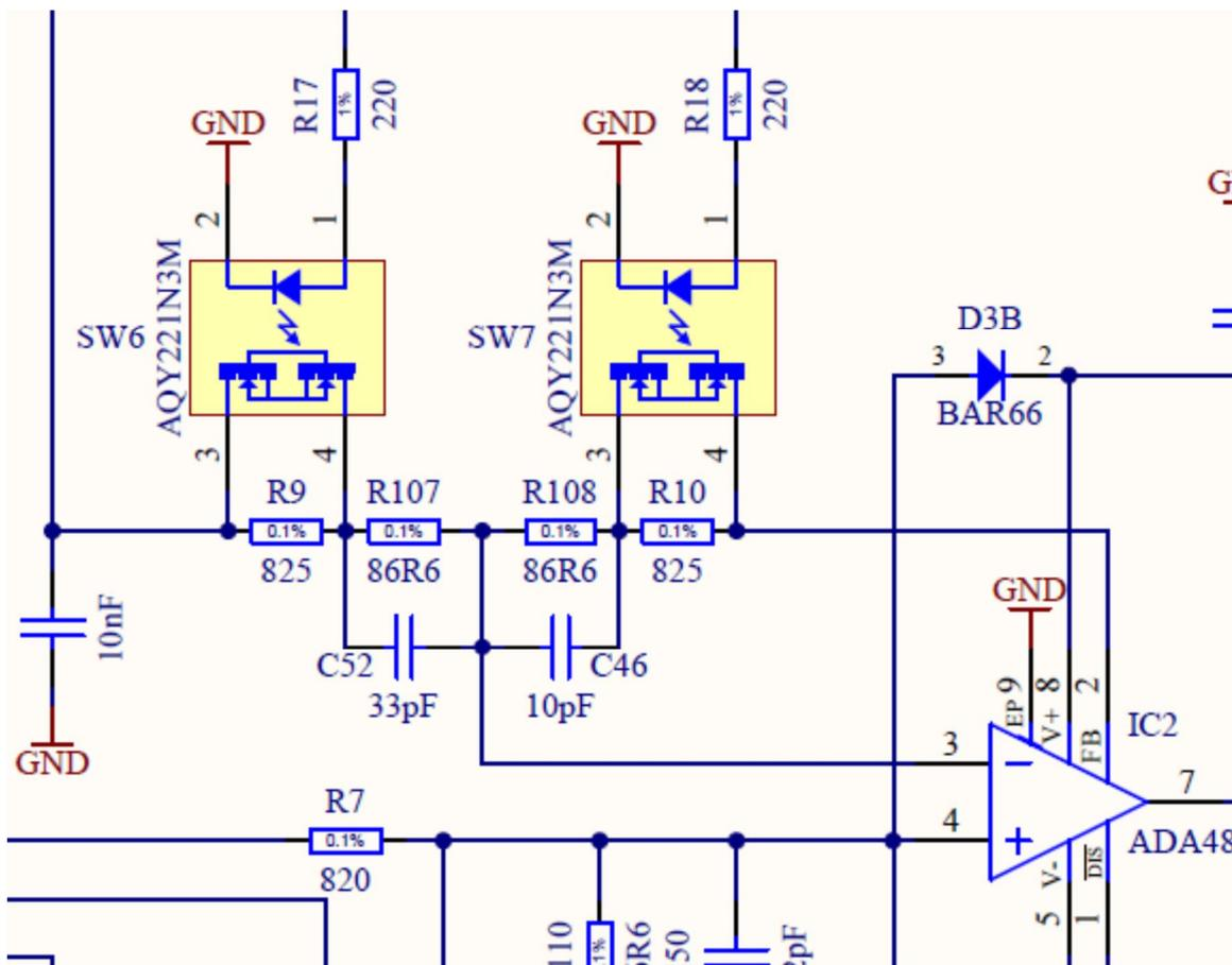
Figure 4: Partial schematic of Channel1
