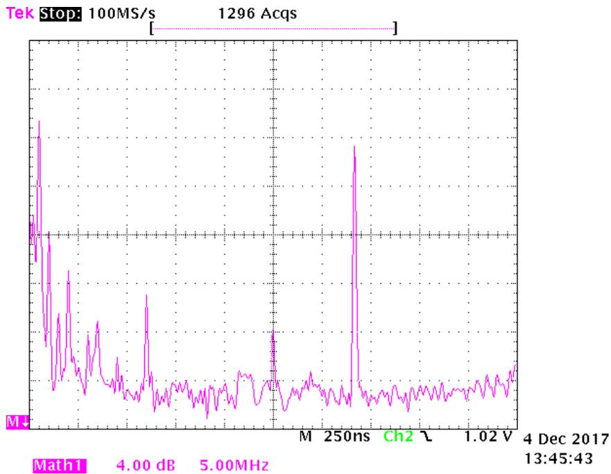
Figure 2: FFT of RF field adjacent to channel 1
