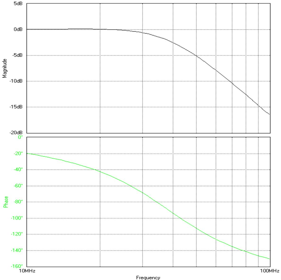
Figure 8: Frequency Response of existing output filter
