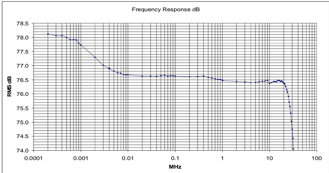
Figure 5: Ref 1 RMS dB Magnified Frequency Response of ADC Sn:139 Ch1 +/-0.5V
