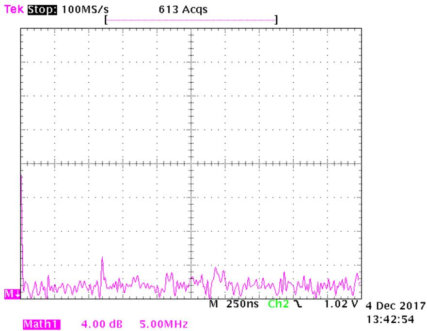
Figure 1: Baseline FFT of RF field outside the PC
