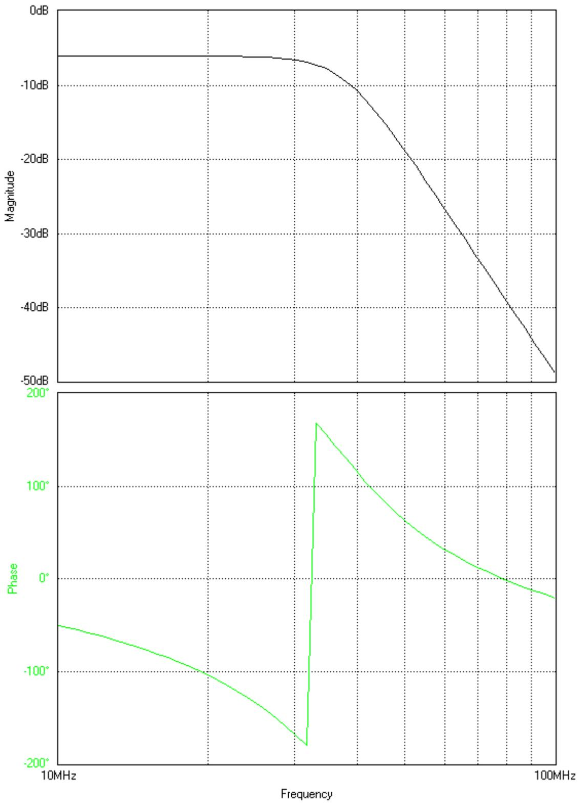
Figure 9: Frequency Response of proposed inter stage filter
