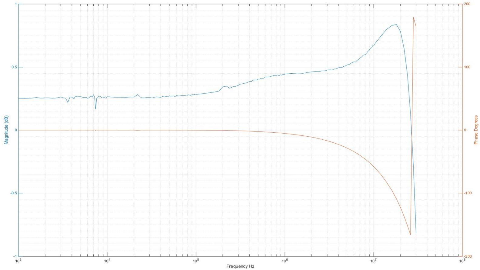
Figure 6: RMS dB Magnified Frequency Response of ADC Sn:139 Ch1 +/-0.5V
