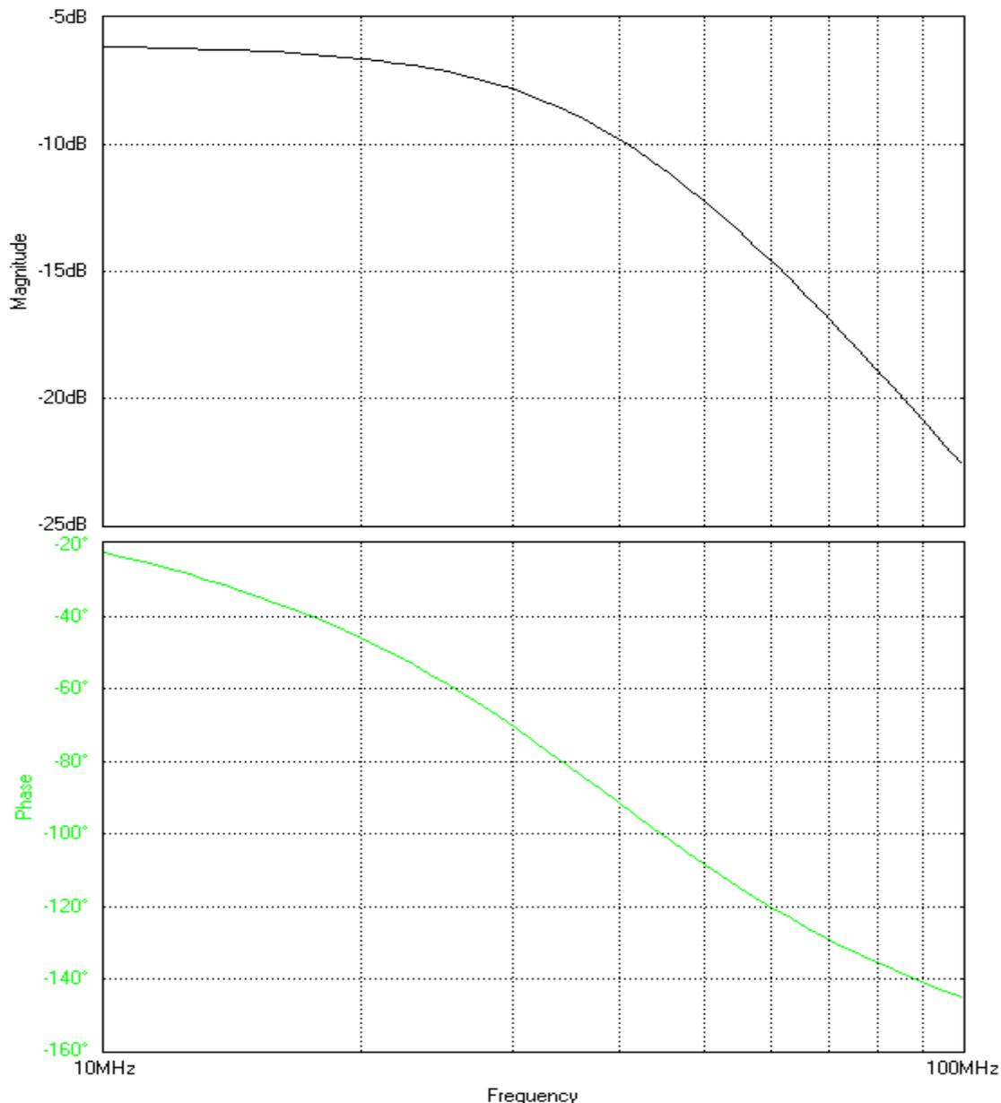
Figure 7: Frequency Response of existing inter stage filter
