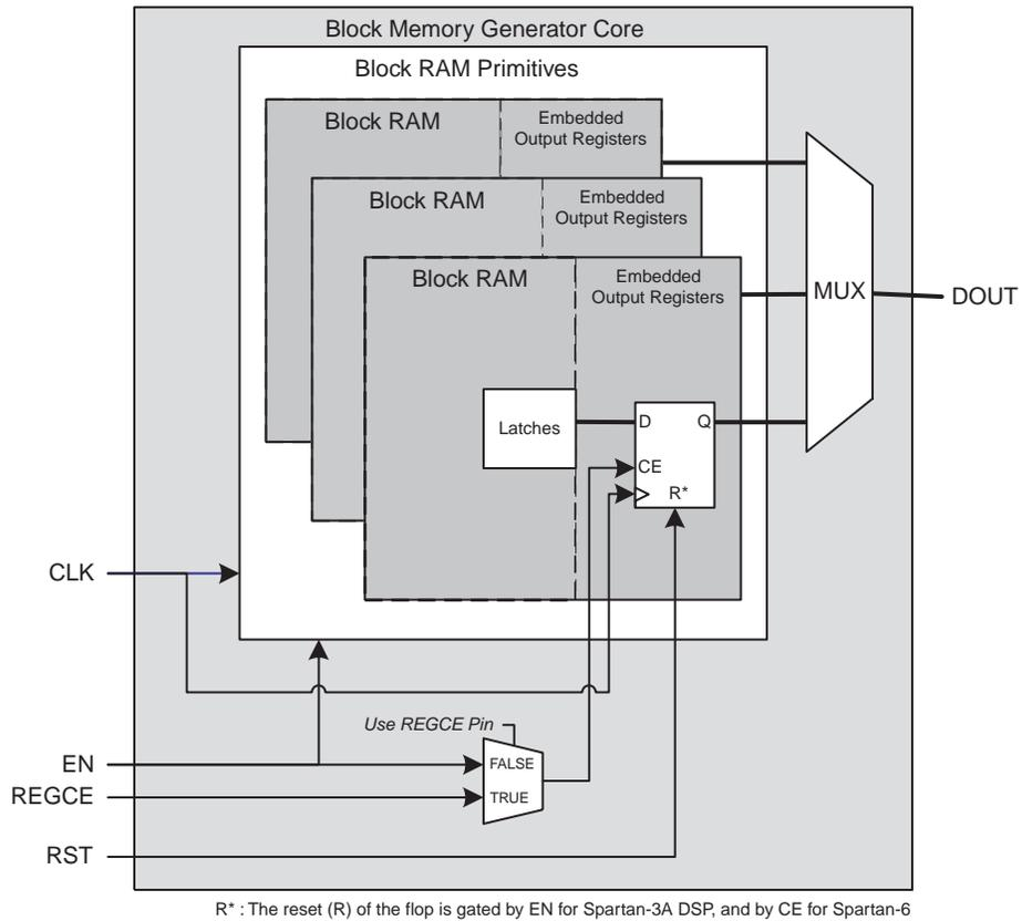
**Figure 75: Spartan-6 or Spartan-3A DSP Block Memory Generated with Register Port [A|B] Gated by EN in Spartan-3A DSP and by CE in Spartan-6 Output of Memory Primitives, Use RST[A|B] Pin Options (With RST), and Special Reset Behavior Enabled**
