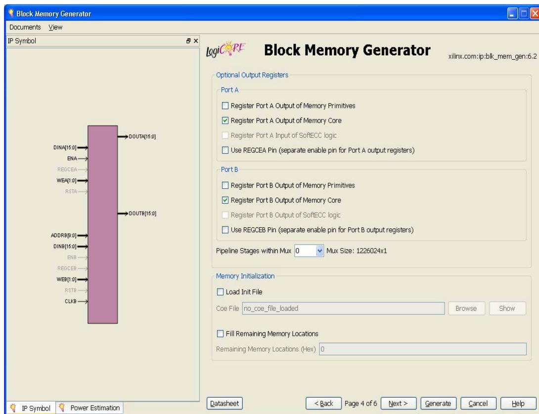
Figure 63: Optional Output Registers Section
