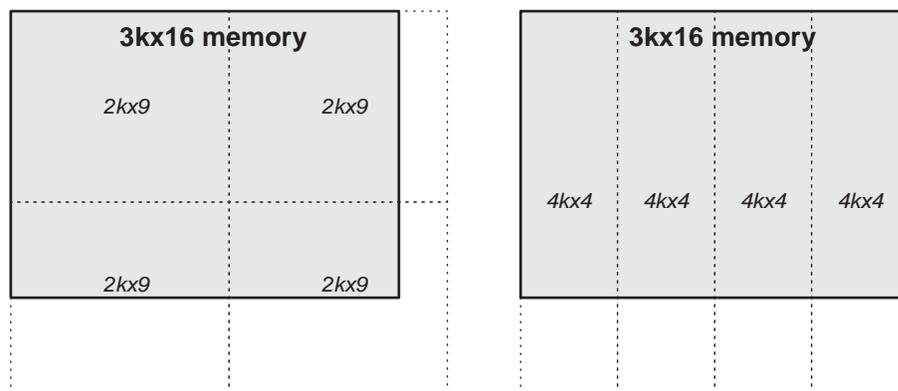
Figure 25: Examples of the Fixed Primitive Algorithm
