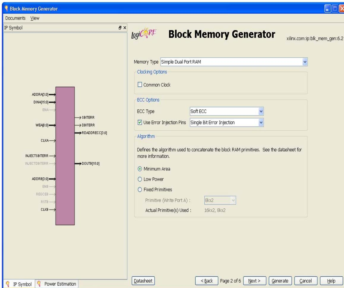
Figure 49: GUI Page 1: Enabling Soft ECC Option
