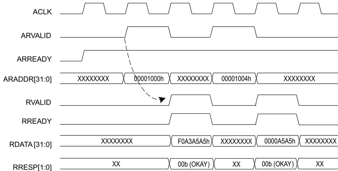
Figure 10: AXI4 Lite Single Burst Read Transactions
