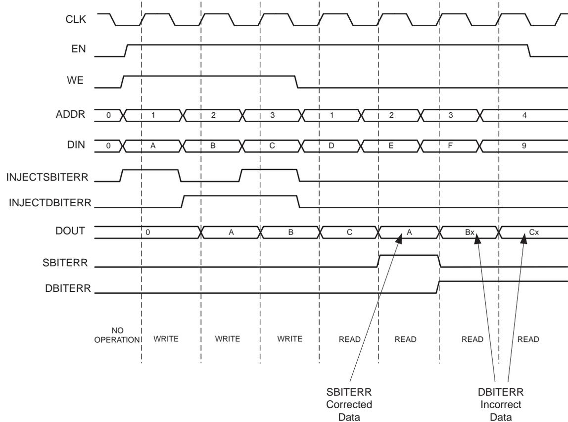
Figure 52: Assertion of SBITERR and DBITERR Signals
