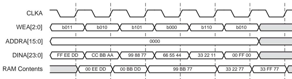
Figure 31: Byte-Write Example
