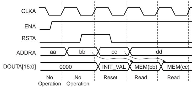
Figure 41: Standard Reset Behavior Similar to Previous Architectures
