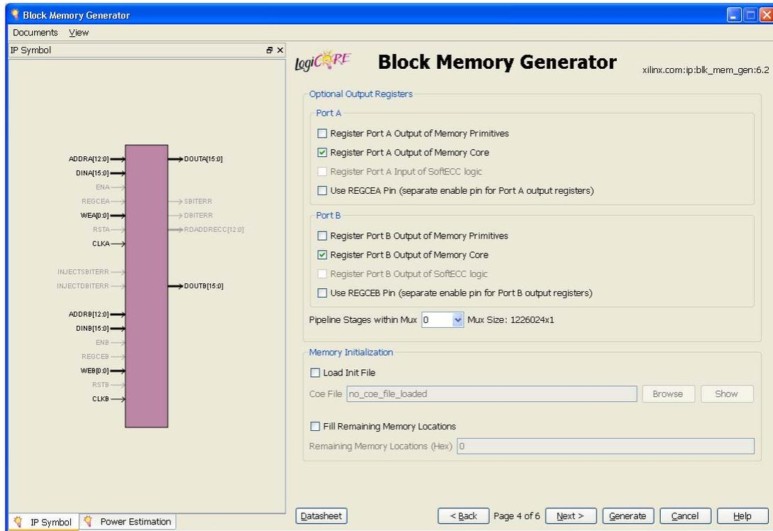
Figure 56: Output Registers and Memory Initialization Screen
