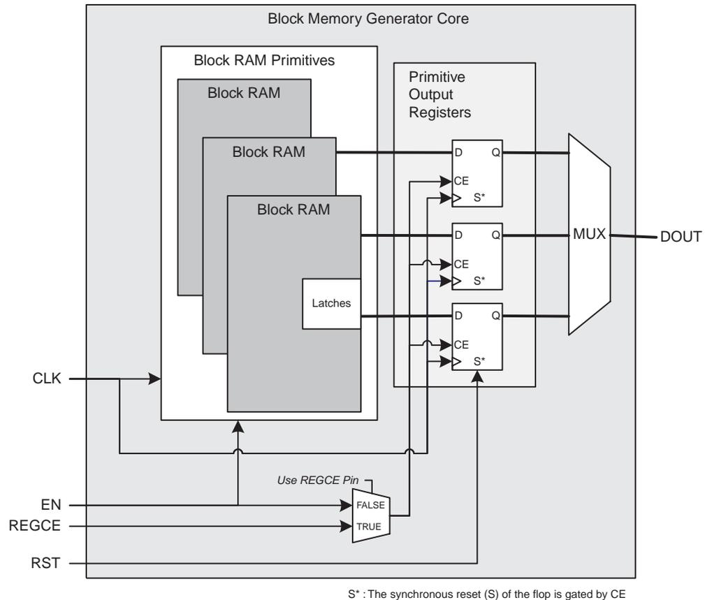
S\* : The synchronous reset (S) of the flop is gated by CE
