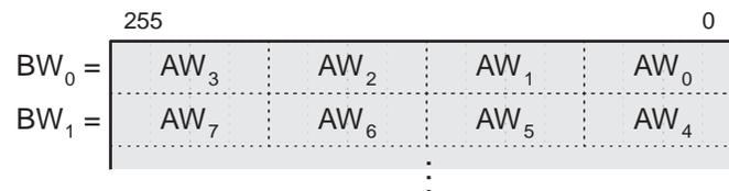
**Figure 30: Read-to-Write Aspect Ratio Example Memory Map**
