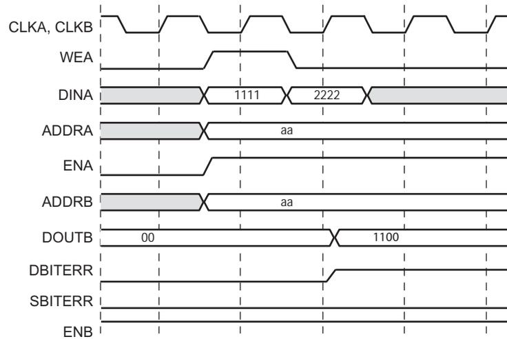
Figure 51: Read and Write Operations with Soft ECC
