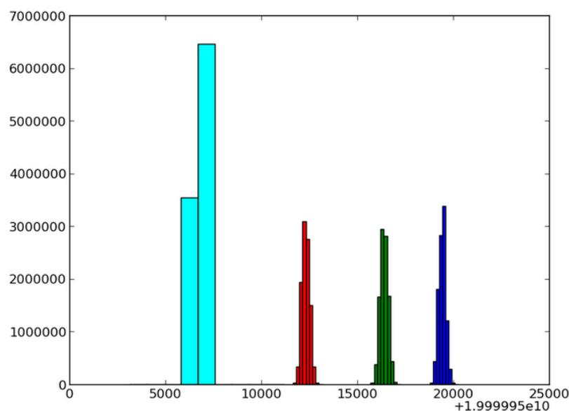
Figure 9: Histograms of the measurements from the four channels without outliers. The same number of bins has been used; cyan measurements are concentrated into fewer bins. Note that because of computation resources issues the graph contains 6M data per channel, rather than 20M.
