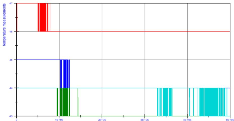
Figure 11: Rough temperature measurements from the One Wire thermometer on each board
