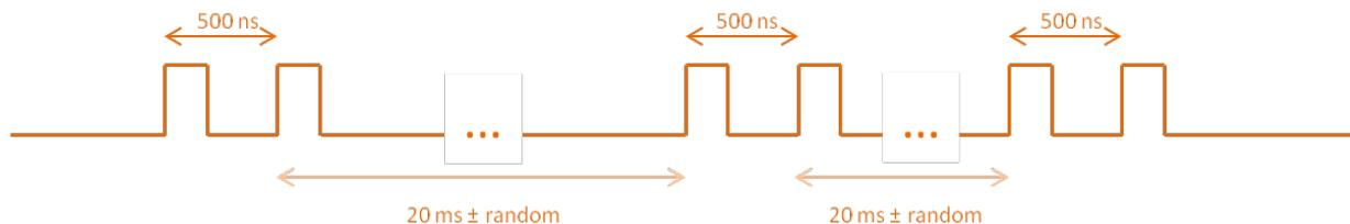
Figure 2: Pulses fed to the TDC boards
