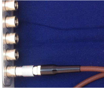
Figure 5: LEMO-00 connector plugged in the first FMC-DIO-5chTTLa-board port (port 0)
