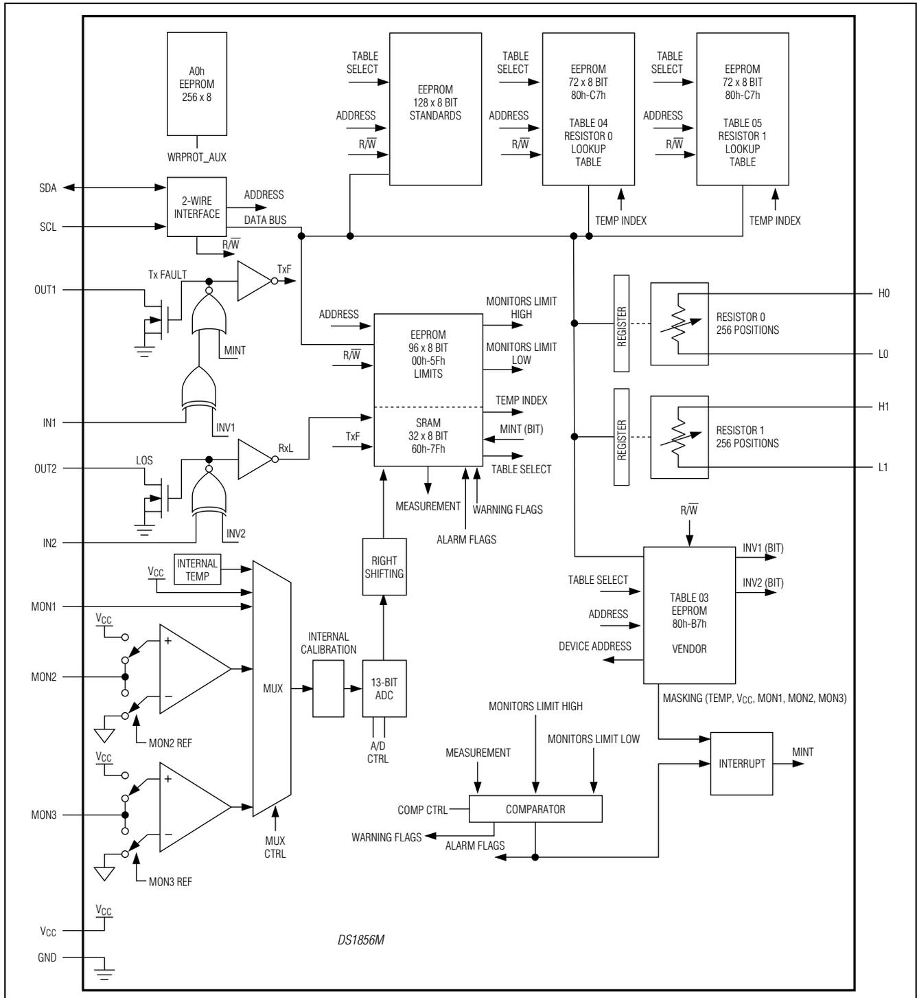
Figure 1. Block Diagram
