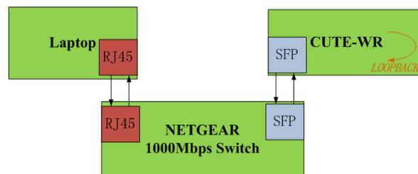
Fig. 5. Ethernet loopback test setup
