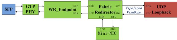
Fig. 6. Ethernet data path in WRPC
