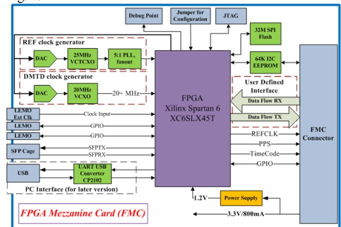
Fig. 1. The CUTE-WR hardware block diagram
