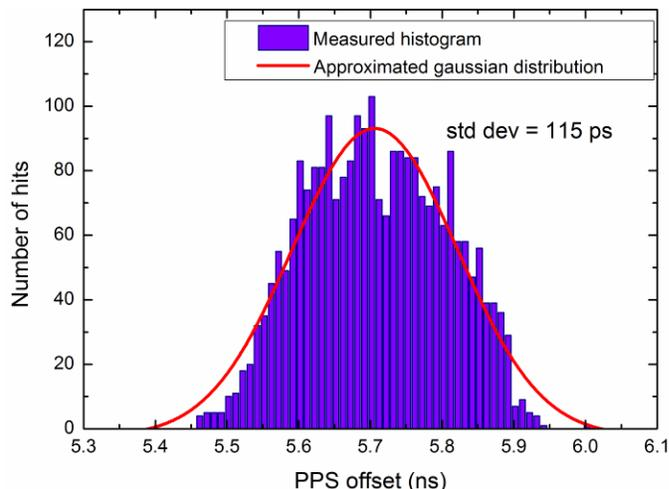
Fig. 4. Measured histogram of PPS offset between SPEC and the WR switch
