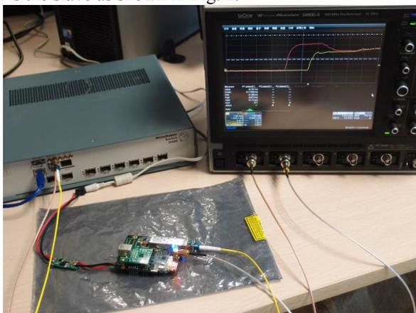
Fig. 2. Time synchronization test setup
