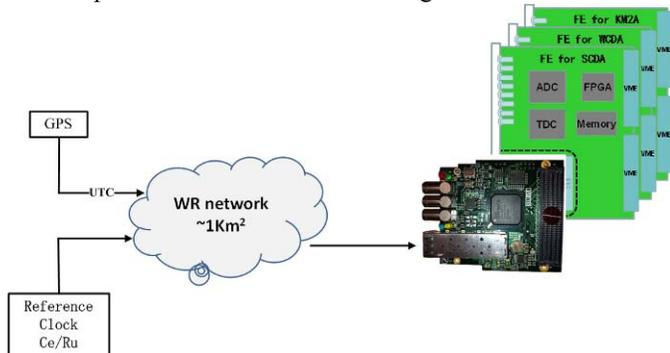
Fig. 7. Clock synchronization architecture for LHAASO. KM2A, WCDA and SCDA are detector arrays in LHAASO project.
