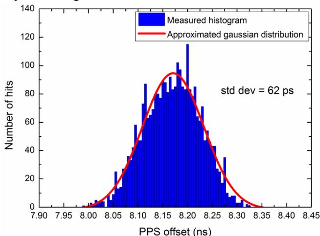
Fig. 3. Measured histogram of PPS offset between the CUTE-WR and the WR switch
